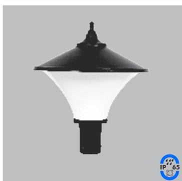
Post top fixture for pole mounted application. Aluminium housing with corrosion resistant powder coat and UV stabilised vandal proof clear diffuser. IP65 protection suitable for outdoor application.
