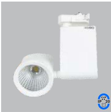
Organic design with die cast housing & heat sink for efficient heat dissipation. Ideal for retail & hospitality. Curved deep diamond facet reflector with glass to cut glare. Optical and thermal solution for high performance.
