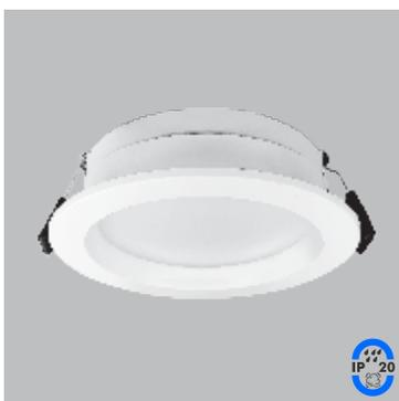
Sleek round backlit LED down light made up of die-cast housing & light weight plastic trim which is designed as a reflector to give high lumen efficacy. Also opal PMMA diffuser is so fixed in inner periphery of trim to cut down the glare & provide uniform light output.
