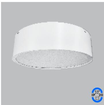
Round luminaire aluminium, rolled profile, seamlessly welded housing with integrated tool-less suspension height adjustment. Highly reflective coating for improved efficiency with high transmission factor PMMA diffuser. Rolled aluminium frame accessory along with fixture for ease in installation.
