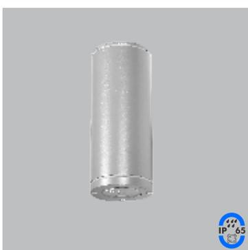
Ceiling mounted IP 65 luminaire made of high grade aluminium extrusion & die cast aluminium heatsink for effective heat dissipation with high efficient COB for better output. The luminaire is available in different beam angles with toughened glass.
