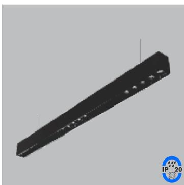
The suspended aluminum extrusion with three reflectors module optics that offers improved efficiency with focus on reduced UGR. Various customisation available with prismatic lens in cell louvers gives flexible light option to the product.
