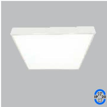
Recessed LED 2x2 luminaire made up of extruded aluminium to give a full glow effect with PMMA low glare diffuser and high efficient LED.
