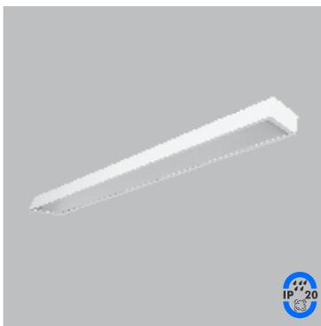
Luminaires compatible with armstrong TECHZONE ceiling. Recessed single length individual luminaire, aluminium extruded natural anodised housing with matt finish extruded PMMA opal diffuser with uniform light distribution.
