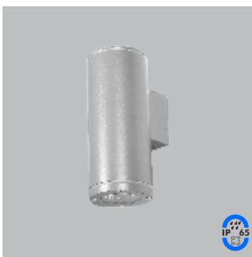
Wall mounted IP 65 luminaire made of high grade aluminium extrusion & die cast aluminium heatsink for effective heat dissipation with high efficient COB for better output. The luminaire is available in different beam angles with toughened glass.
